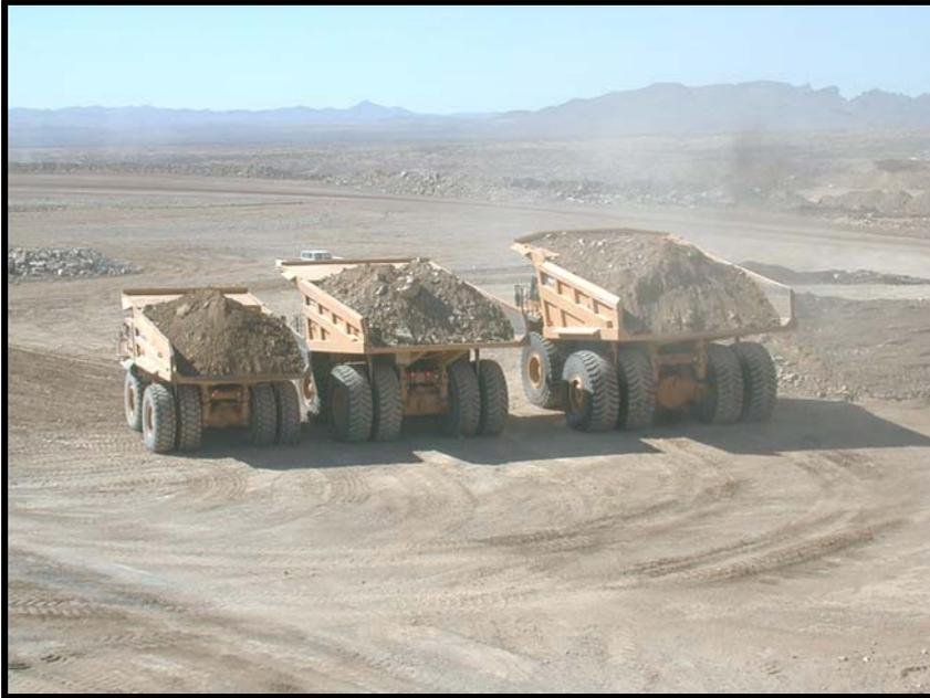
**Photograph 4 – Truck and tire width comparison – 150 vs. 220 vs. 325 tonne class**
