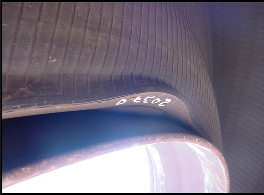
Photograph 11 – Distorted tire bead resulting from imperfect rim mounting
