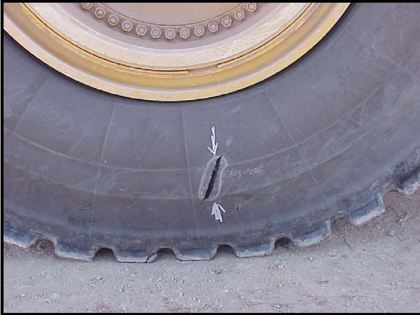
**Photograph 3 – Sidewall damage (55/80R63)**
