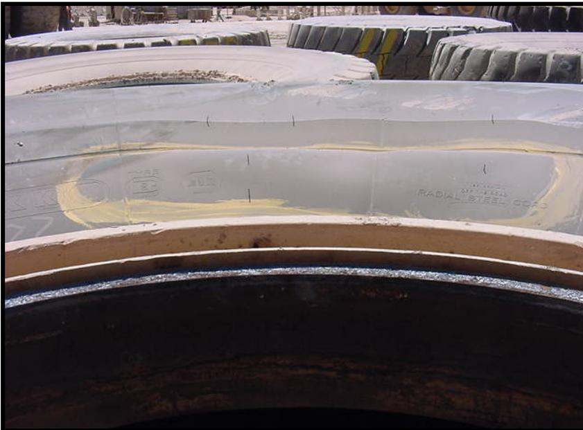
Photograph 12 – Sidewall separation resulting from distorted bead
