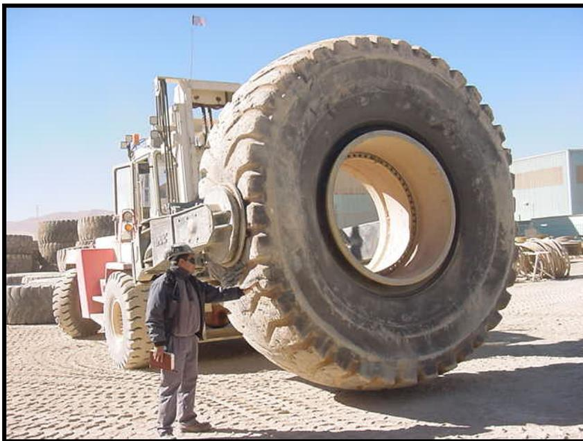
**Photograph 8 – 13.5 tonne lift tire manipulator with 55/80R63 tire**
