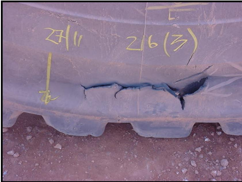
**Photograph 2 – Mechanical separation of the tire shoulder (55/80R63)**
